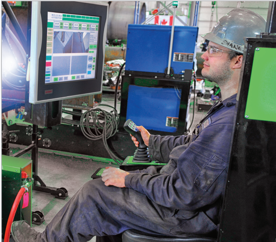
ProStar welding gantries are built with the user in mind. An intuitive touchscreen HMI with aviator style joystick easily control all gantry functions. Set low to the floor, a moving, high-back operator's seat offers comfort and safe proximity to the work area.
