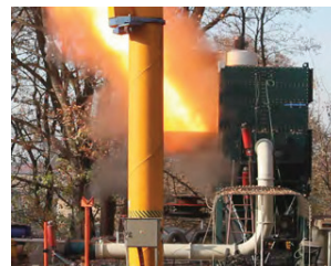
The flame is diverted away from the dust collector to a safe area.
