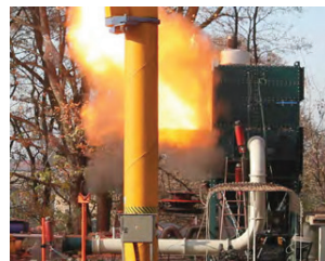
Approximately 50 milliseconds later, the dust ignites and the vent opens.
