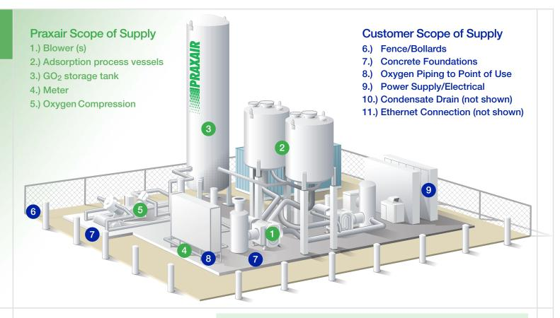
For customers needing up to 95 tons per day of oxygen, the ideal supply is Praxair's VM62 S-XL. The VM62 S-XL is a vacuum pressure swing adsorption (VPSA) plant that consists of a feed blower, sieve beds, vacuum blowers, surge tank and silencers. The system is designed and shipped on three skids - allowing very rapid field installation and minimum disruption to your site. Product delivery pressure is tailored to each customer's unique requirement.
