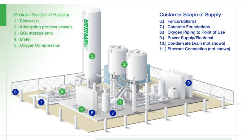
For customers needing up to 190 tons per day of oxygen, the ideal supply is Praxair's VM-120 S-L. The VM-120 S-L is a vacuum pressure swing adsorption (VPSA) plant that consists of a feed blower, sieve beds, vacuum blowers, surge tank and silencers. The system is designed and shipped on five skids allowing very rapid field installation and minimum disruption to your site. Product delivery pressure is tailored to each customer's unique requirement.
