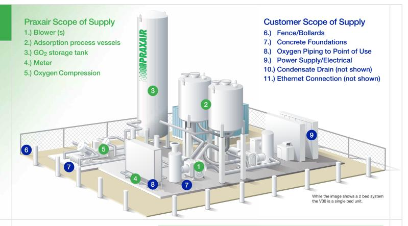
For customers needing up to 36 tons per day of oxygen, the ideal supply is Praxair's V30C. The V30C is a vacuum pressure swing adsorption (VPSA) plant that consists of a feed blower, sieve bed, vacuum blower, surge tank and silencers. The system is designed and shipped on two skids – allowing very rapid field installation and minimum disruption to your site. Product delivery pressure is tailored to each customer's unique requirement.
