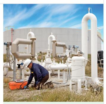
The *Tracer Tight* service is used by most petrochemical companies in North America because it is one of the most sensitive testing methods, compatible with site operations and it locates leaks without ever taking tanks or pipelines out of service.
