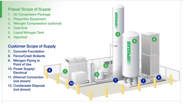
For customers needing up to 108,200 cfh-ntp of nitrogen, the ideal supply is Praxair's N80. The N80 is a cryogenic nitrogen plant that consists of a **Warm End** which includes the air compressor package and prepurifier equipment, and a **Cold End** which includes the distillation column, primary heat exchanger, and main condenser. The N80 uses liquid assist for the refrigeration requirement of the plant. The system also comes with a liquid nitrogen **Backup System** for ultimate reliability.
