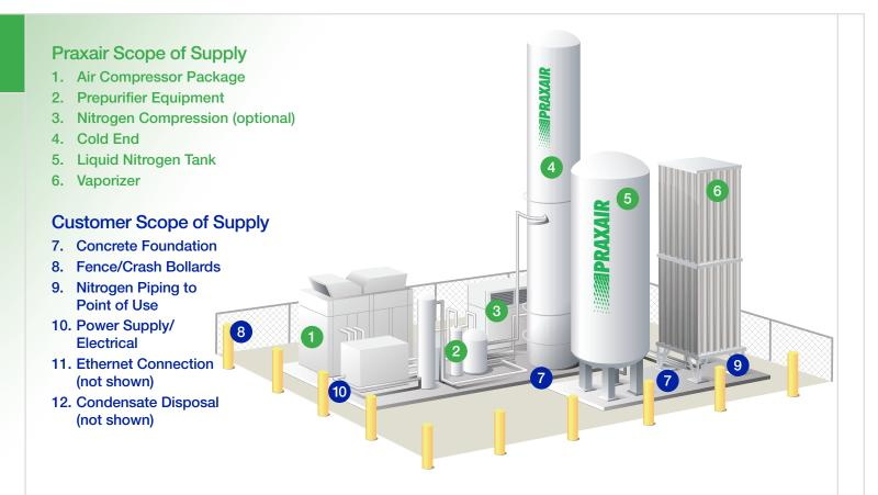
For customers needing up to 45,100 cfh-ntp of nitrogen, the ideal supply is Praxair's N30. The N30 is a cryogenic nitrogen plant that consists of a **Warm End** which includes the air compressor package and prepurifier equipment, and a **Cold End** which includes the distillation column, primary heat exchanger, and main condenser. The N30 uses liquid assist for the refrigeration requirement of the plant. The system also includes a liquid nitrogen **Backup System** for ultimate reliability.
