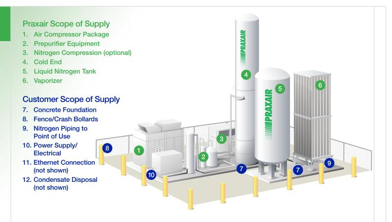
For customers needing up to 17,700 cfh-ntp of nitrogen, the ideal supply is Praxair's N10. The N10 is a cryogenic nitrogen plant that consists of a **Warm End** which includes the air compressor package and prepurifier equipment, and a **Cold End** which includes the distillation column, primary heat exchanger, and main condenser. The N10 uses liquid assist for the refrigeration requirement of the plant. The system also comes with a liquid nitrogen **Backup System** for ultimate reliability.
