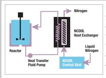
non-freezing injector to achieve maximum cooling efficiency. Injecting the liquid nitrogen directly into the process fluid or reactants achieves fast response and precise temperature control required for fine chemical applications. The proprietary injector is a critical component as it eliminates the freezing risk associated with other direct injection approaches.
